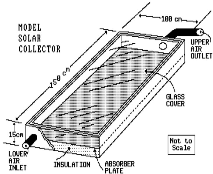
The solar collector is placed outside in sunlight, facing south and tilted  $40^\circ$  from the horizontal. At which position of the Sun would the collector receive the most intense solar radiation?
